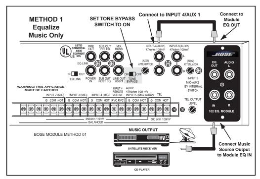
Fig. 26 - Method 1 Module Wiring Diagram
